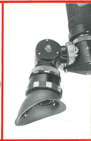
This is the position of the periscopic finder attachment for viewing with the left eye when the 400 ft (120 m) magazine is in position.
